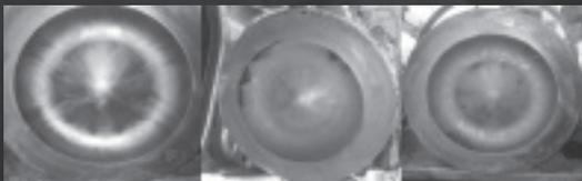
*"...these pistons are just as they came out of the engine which has over 860,000 KM on it. The mechanic stated he has not seen an engine burn so clean. You can see the spray pattern the top of the pistons."*
